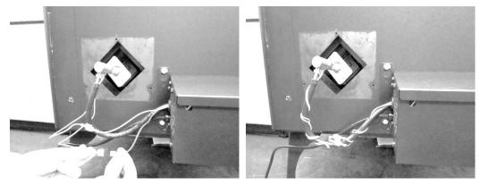
8. Attach the cover box to the heat shield as shown below, using the screws removed in step 2. If your unit does not include these holes, drill the holes with the included bit.
