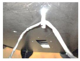
11. Push any excess start switch wiring into the compressor assembly. NOTE: A lock-tie is included to secure excess wiring.
