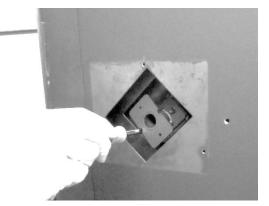
5. Attach the igniter with gasket to the igniter sleeve using the screws and gasket included in this kit. Note that the igniter gasket is placed between the sleeve and igniter assembly.
