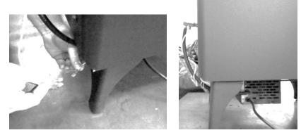
13. Attach the igniter switch to the bottom of the stove using the 10-24 x  $\frac{1}{2}$ " screws provided, as shown below.
