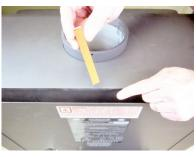
4. Remove the backing from the silicone gasket.
