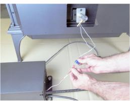
11. Attach the ¼" tube to the nipple on the igniter.
