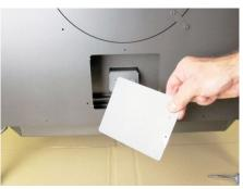
6. Remove the igniter cover plate and gasket. Retain the gasket and screws.
