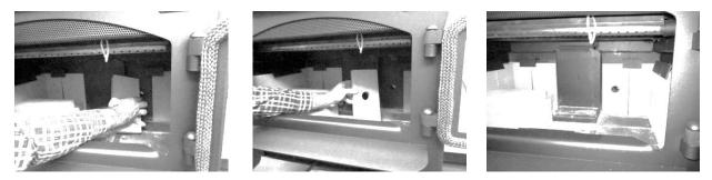
2. Remove the cover plate from the rear of the stove as shown below. Retain the screws.
