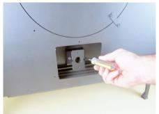
8. Attach the igniter with gasket to the igniter sleeve using the screws and gasket included in this kit. Note that the igniter gasket is placed between the sleeve and igniter assembly.
