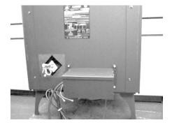
3. Tighten the bolts to secure the compressor assembly to the stove. A ratchet with an extension may help with this task.
