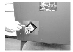
NOTE: These instructions show the compressor assembly attached to the back of the stove. Alternatively, you may place it on the floor near the stove. See the Cape Cod model installation instructions on page 12 for details.
