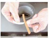
5. While pushing the heat shield back, insert the gasket between the heat shield and heat shield support. Affix the gasket to the heat shield. The photo at right below shows the gasket properly placed.
