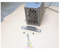
d. Install 2 grommets (both sides) into the foot plates.
